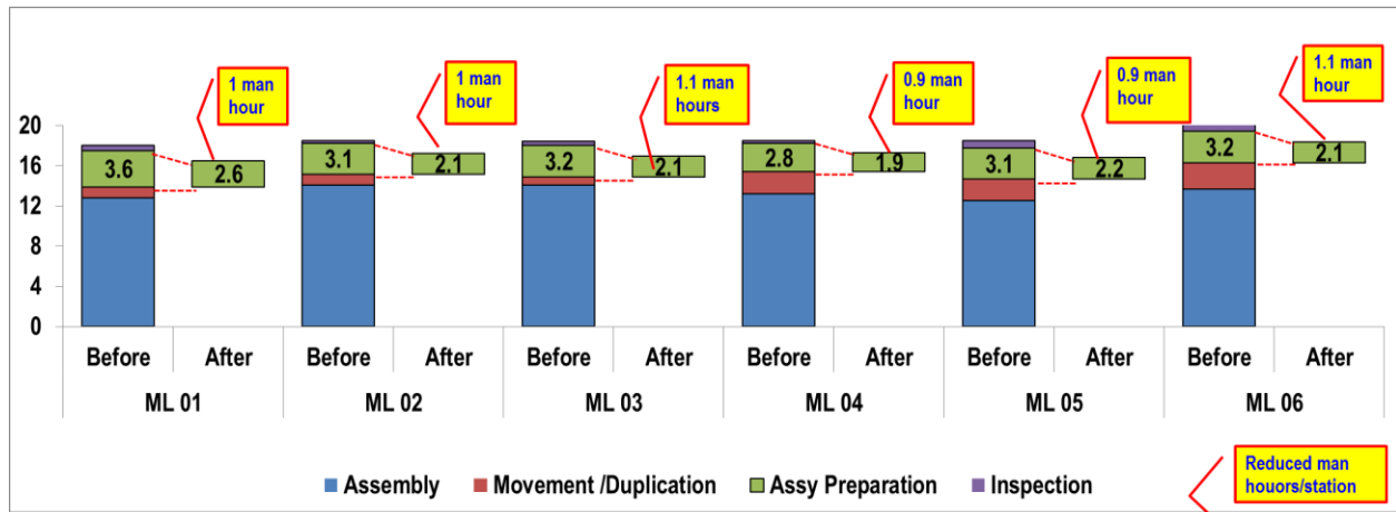
Chart 8.3.1 Effect of Muda on reduction of man hours in assembly preparation process
